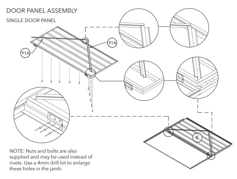
NOTE: The holes to fasten the padbolt hasp are not pre-punched to allow for proper alignment. Position the hasp centrally over the padbolt shaft and drill 3mm holes and secure with screws.
