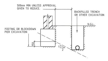
The contactor shall undertake investigatory localised excavations near existing footings to ascertain their depth prior to excavating adjacent to them. It is noted that excavating to a depth below that indicated above shall not be undertaken without the written approval from the engineer.
