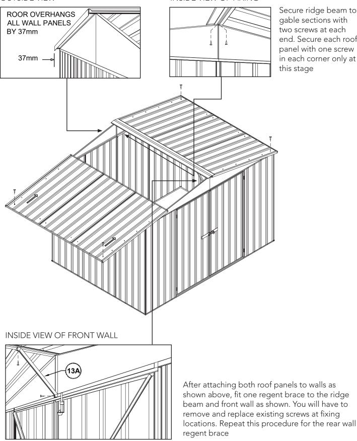
Secure ridge beam to gable sections with two screws at each end. Secure each roof panel with one screw in each corner only at this stage
