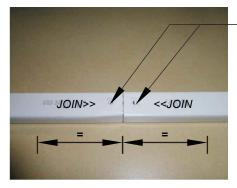
Finished Channel. The joined channels should now look like the picture with the CSJ positioned equally inside of the joined channels.
