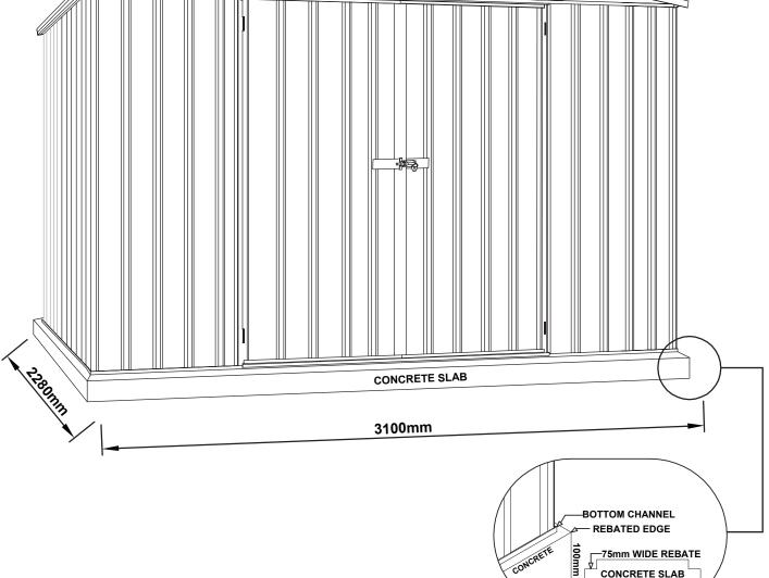
For construction in non-cyclonic areas Wind rating: N2 as per AS4055-2012. If you require a higher wind rating please contact us: admin@absco.com.au or 1800 029 701
