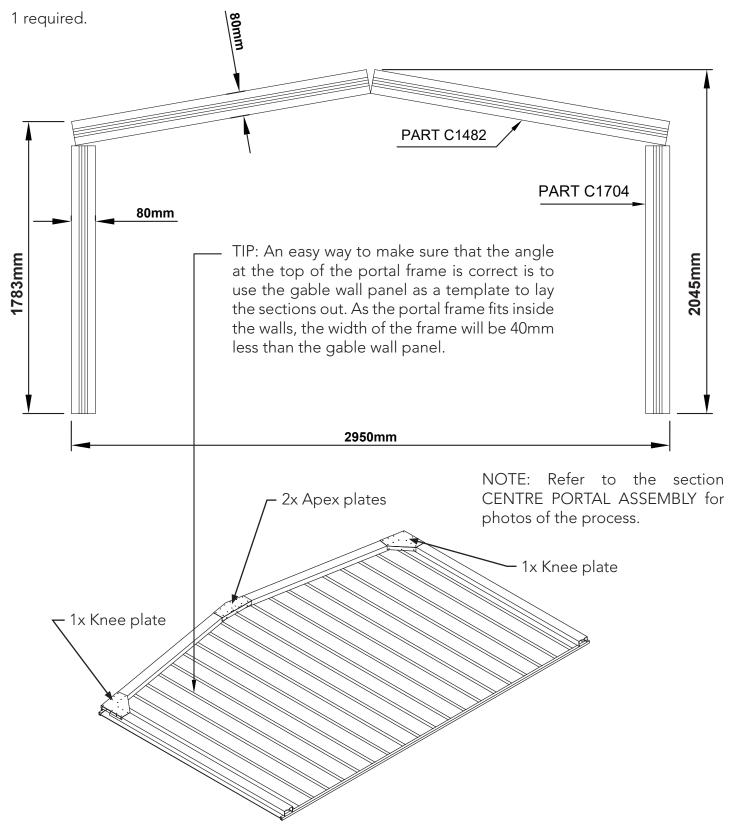
NOTE: If you have a slab with an edge rebate in your concrete slab, you will have to cut an amount off the bottom of the frame legs equal to the depth of the rebate.
