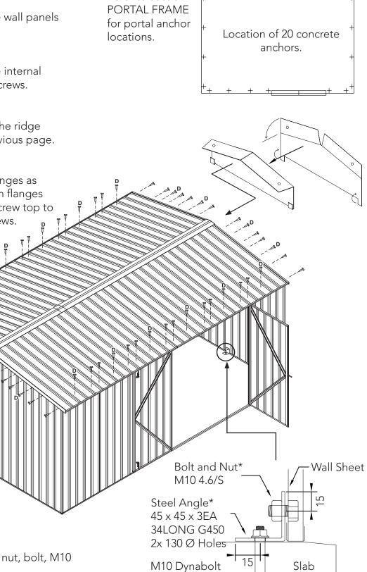
Each anchor consists of one nut, bolt, M10 dynabolt and steel angle. Drill a 10mm hole into the wall sheet. Drill a 10mm hole into the concrete.
